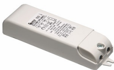
OPTIONAL Power supply RF25747 Power supply 24V 10W /110-240V IP20 Class II selv. Non Dimmable
